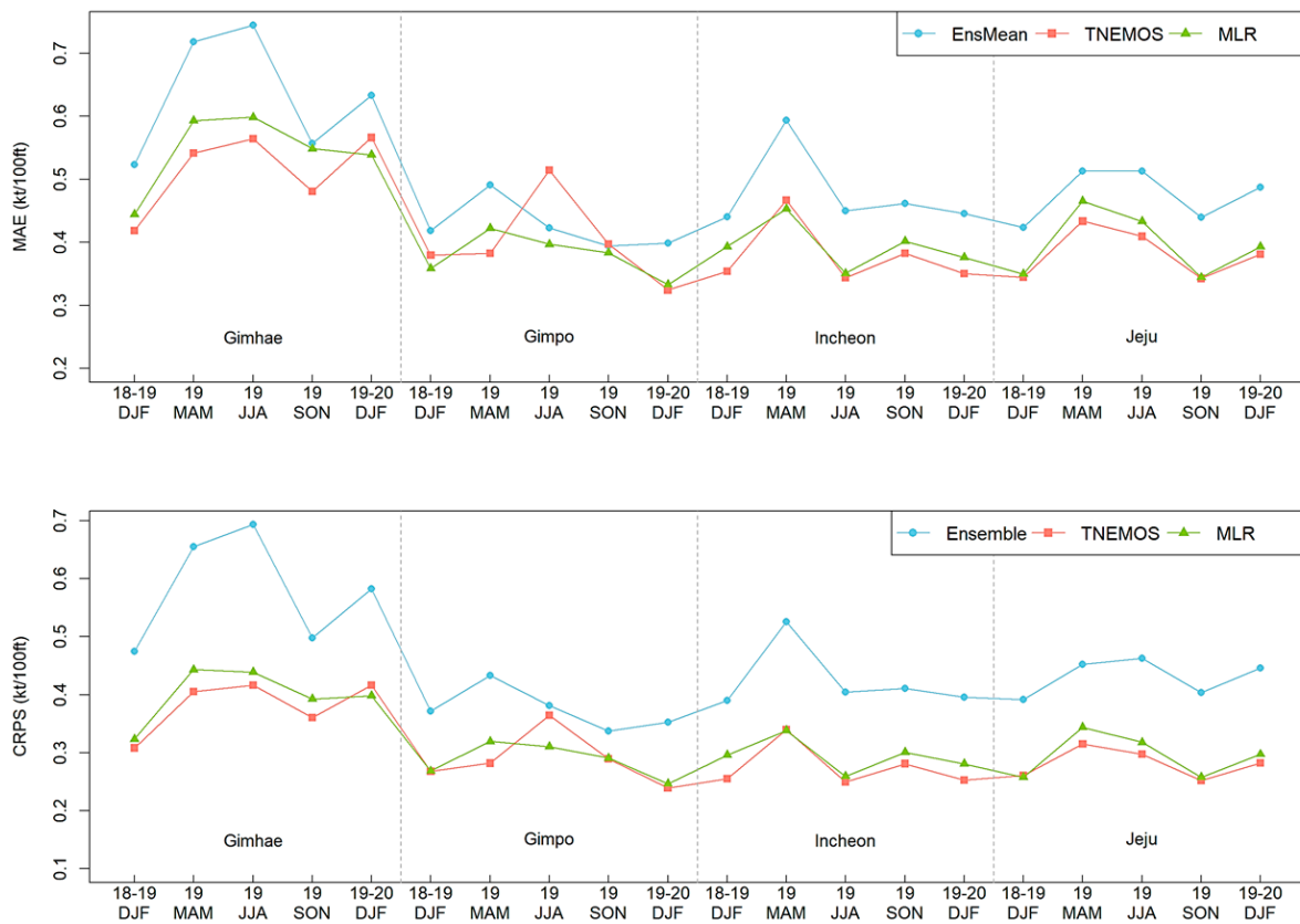
Figure 9. Comparison of prediction errors of ensemble mean, multiple regression and TNEMOS based on test datasets in terms of MAE and CRPS.
